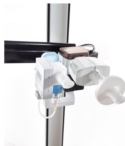
Vyntus™ APS Aerosol Provocation System integrated inside the cabin for automated, software-controlled, safe and accurate bronchial challenge testing
